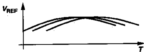
Figure 11.17 Variation of the zero-TC temperature for difference samples.
