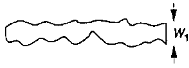
Figure 18.2 Excessive width variation in a narrow poly line.
