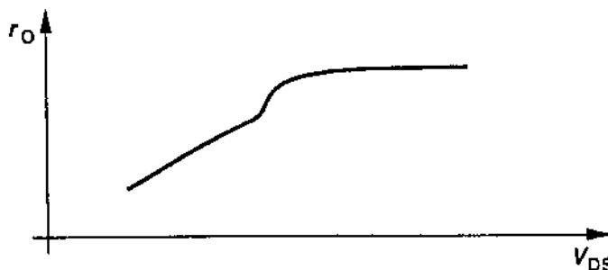
Figure 16.14 Kink in output resistance in Level 3 model.
